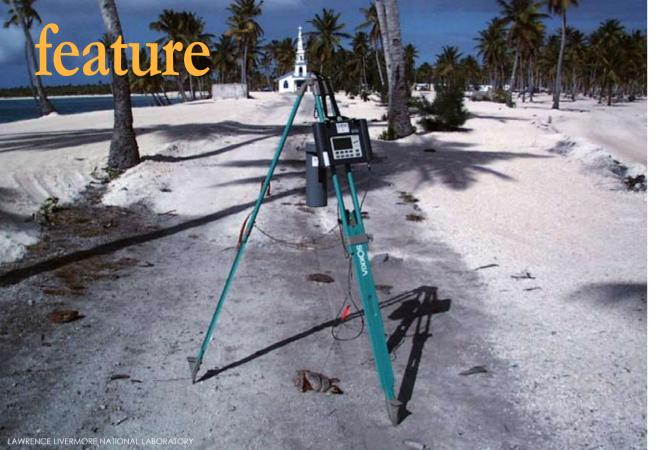
A gamma spectrometer for determination of external gamma exposure rates in village and housing areas where people spend most of their time.
